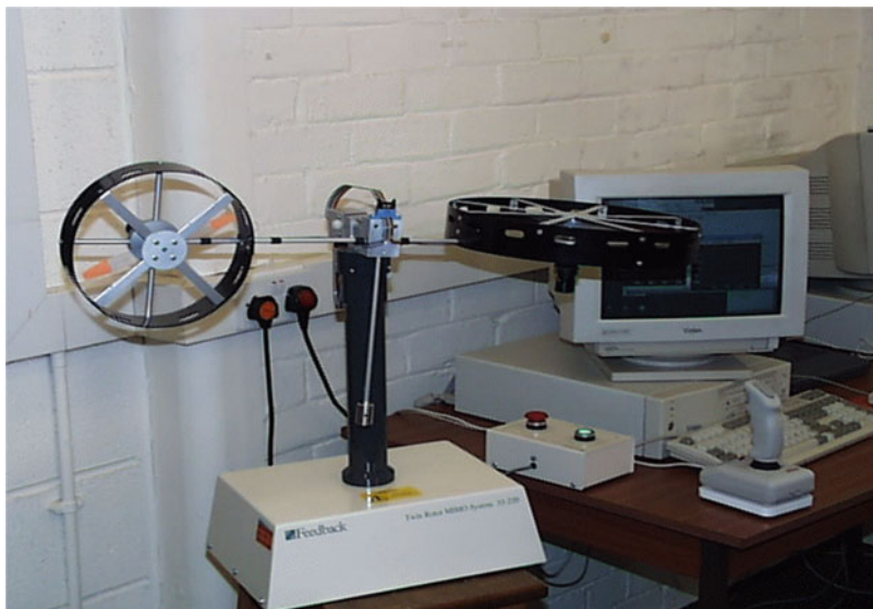
Fig. 8.9 The twin rotor experimental rig used at Sheffield University
